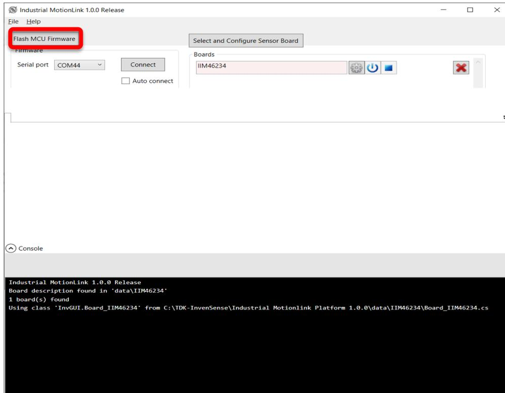
**Figure 18. Flashing the MCU Firmware**
