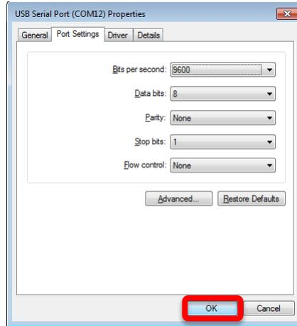
**Figure 33. USB Serial Port Properties**
