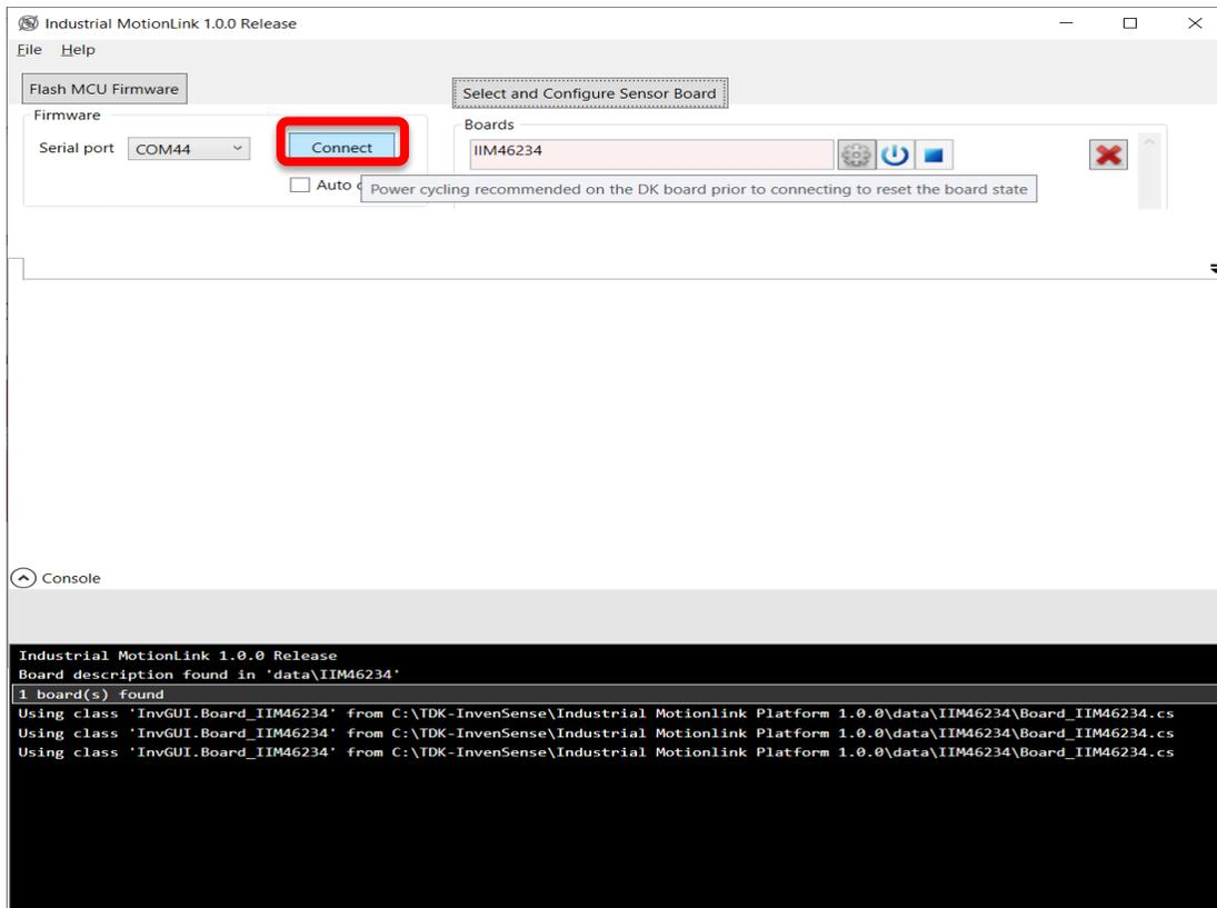
**Figure 22. Connect to the Sensor Board**
