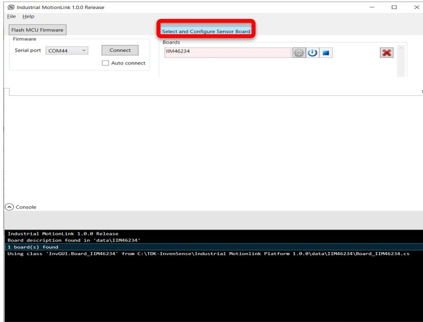
Figure 19. Selecting and Configuring Sensor Board
