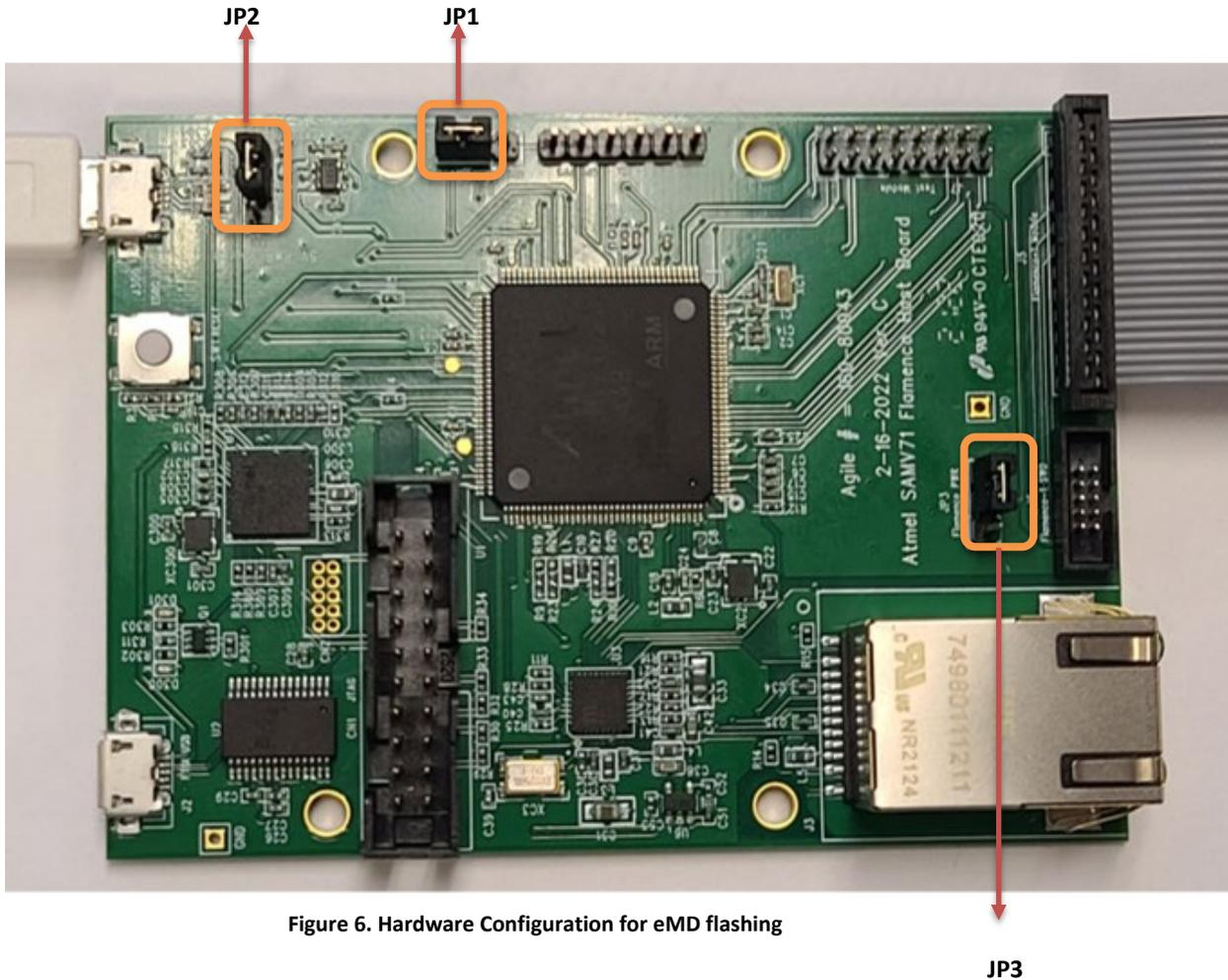
Figure 6. Hardware Configuration for eMD flashing
