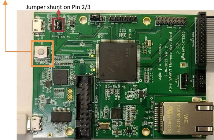
**Figure 4. Software Reset Button**
