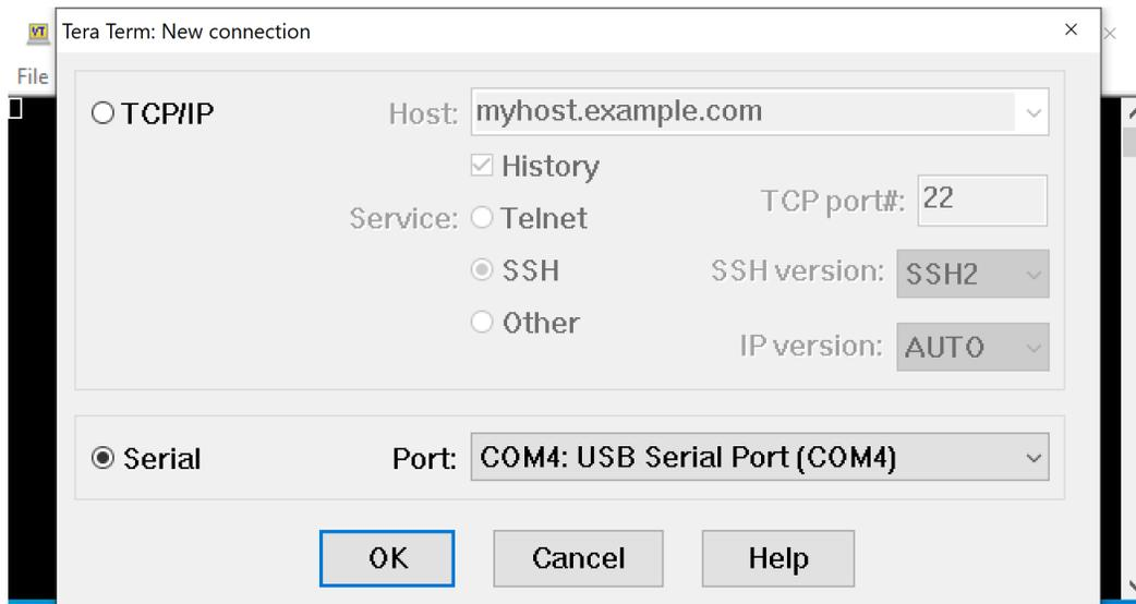
**Figure 2. New Connection Setting**
