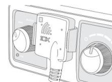
The NFC reader comes with a convenient mounting bracket that can either be screwed in place (screws provided) or taped in place (tape provided).
