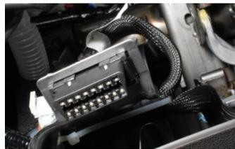
All Geotab devices have a sensitive accelerometer built in, for this to calibrate and work correctly the device **MUST** be secure in vehicle and not be able to move freely
