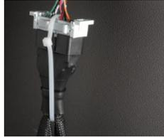
Attach the GO device to the HRN-EUNI securing the connection using a Geotab serialised zip tie. (Supplied with GO9)
