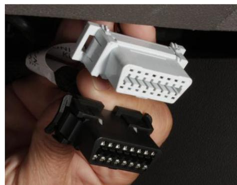
The receiver end of the HRN-EUNI will plug into the original vehicle connector
