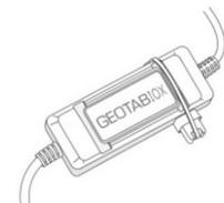
4. Once your connections to the IOX-AUX wiring have been made, connect the GO9 and immediately start the vehicle. The IOX is now in self-learn mode and your GO9 is in debug mode.
