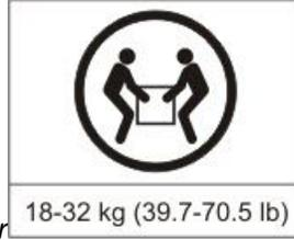
or or The weight of this part or unit is between 18 and 32 kg (39.7 and 70.5 lb). It takes two persons to safely lift this part or unit. (C009)
