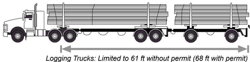
**Only trailer and load constitute regulated length** unless the tractor also carries freight. Single trailers may not exceed 53 feet (56 feet maximum with permit). The legal length of combination vehicles may vary. For example, truck and trailer combinations may not exceed 75 feet. Two trailing units (doubles) may not exceed 61 feet (68 feet maximum with permit).
