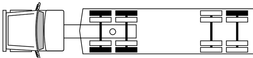
All tires on one drive axle or one tire on each side of both drive axles.
