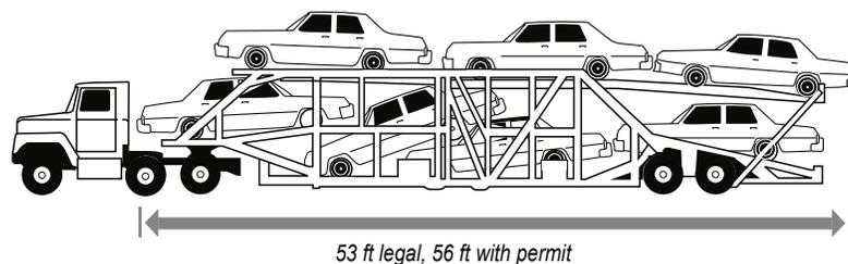
To be considered specialized equipment, the power unit and trailer must both be designed to transport automobiles.
