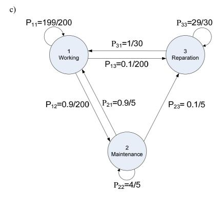
Suppose that there is one jump each day. The sum of all transition probabilities from one state must be equal to 1, including the probability to go back to the same state. From this, the transition probabilities for the generator can be calculated.
