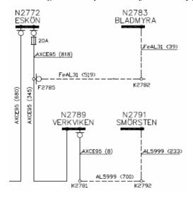
The figure illustrates a small part of a real distribution area at the 10 kV-level. You shall draw up a suitable model of the grid, and then make a few reliability calculations. In order to simplify things, it is supposed that Eskön is connected at a transformer point to a "strong" grid, where the feeding never fails (through the 680 m cable that in the figure ends up in nowhere.)
